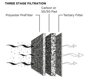
**CarbonWeb** filters utilize 60% activity granular activated carbon (gac) for general odor removal. **CarbonWeb Plus** contain equal volumes of 60% gac and activated alumina impregnated with 5% potassium permanganate to remove odors and light gases. Both products provide a fresher, more odor-free environment.
